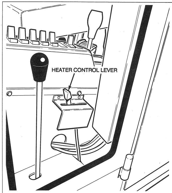
The Heater Control Lever is located on the right-hand side of the cab. Move the lever to increase or decrease the temperature.
